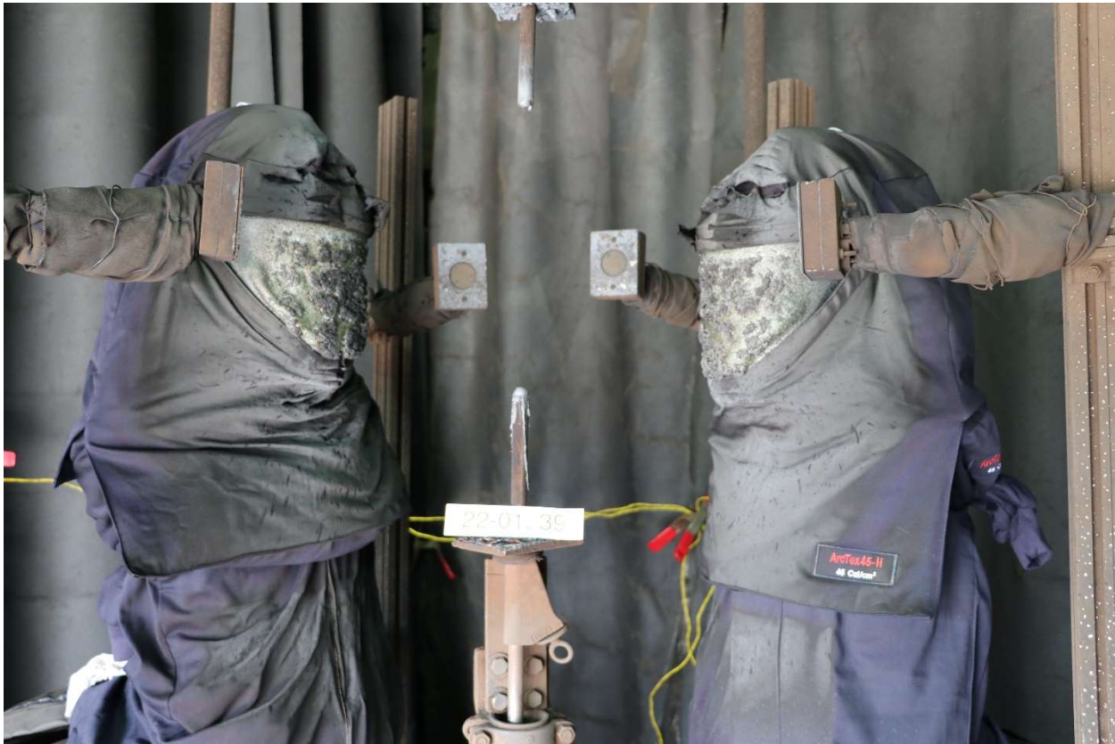
Figure 6-2: Photograph of a specimen after the arc exposure.
