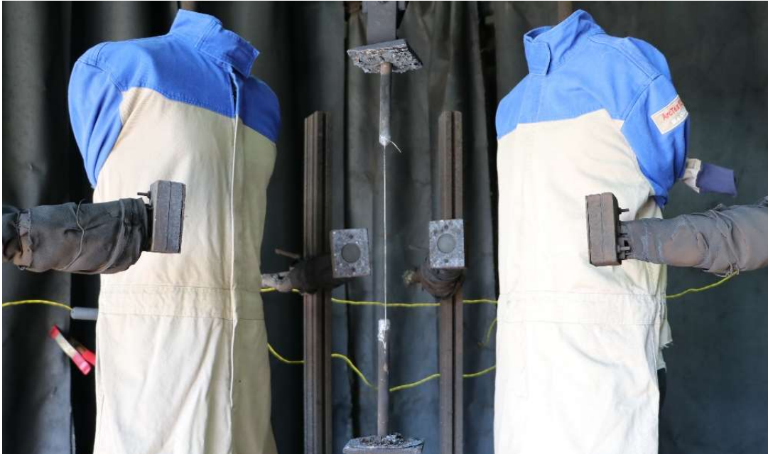
Figure 6.1: Garments as tested before arc exposure.
