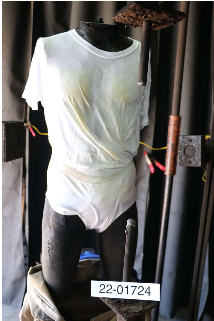
Figure 6.3: Undergarment after arc exposure. (Test# 22-1724)
