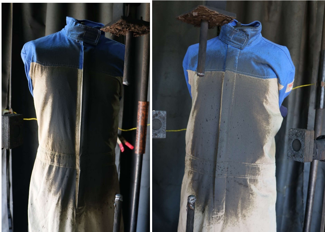
Figure 6.2: Garments after arc exposure. (Test# 22-1724)
