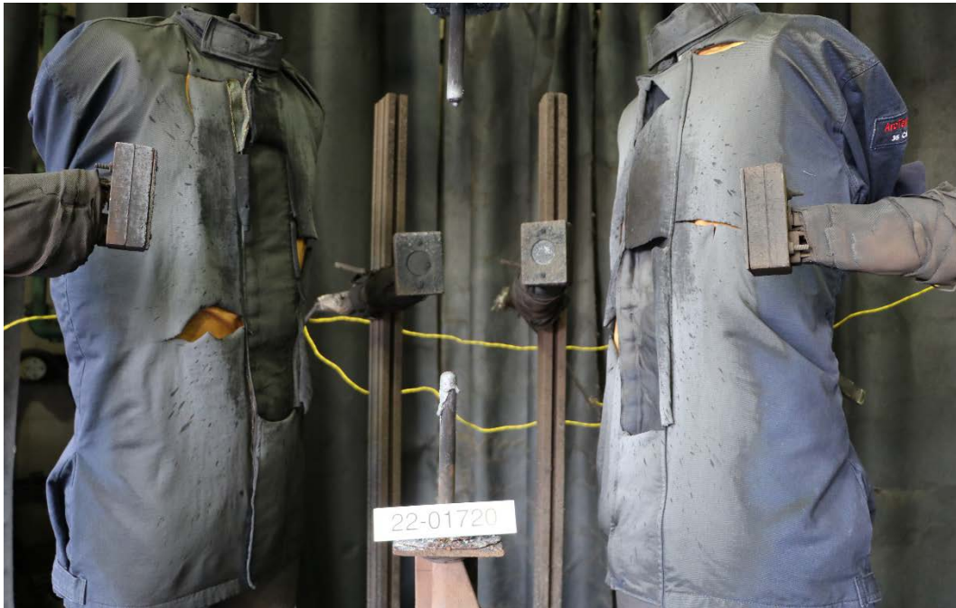
Figure 6.2: Garments after arc exposure. (Test# 22-1720)
