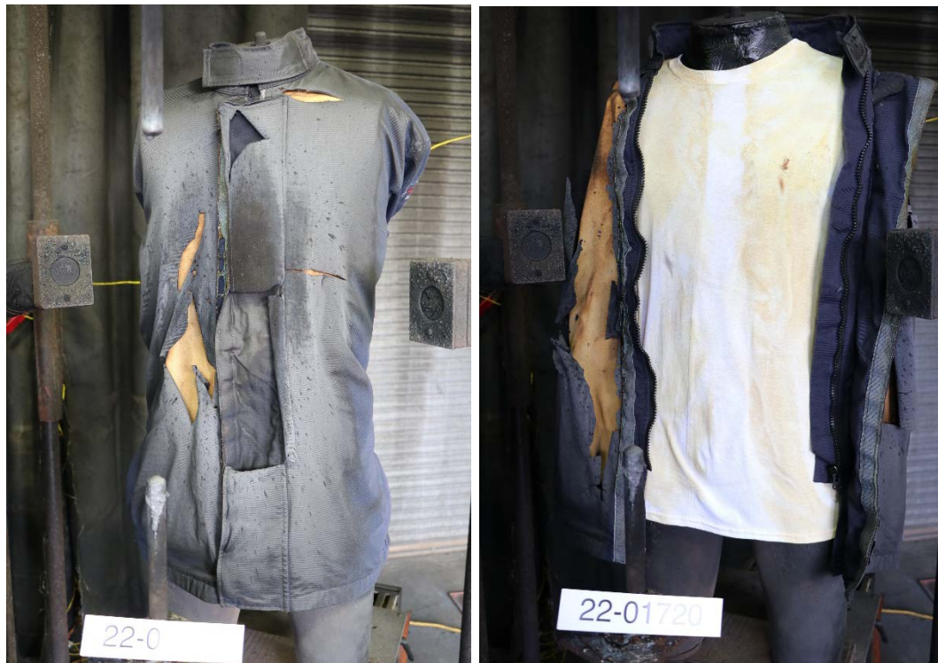
Figure 6.4: Exposure of garment and underlayer garment. (Test# 22-1720B)
