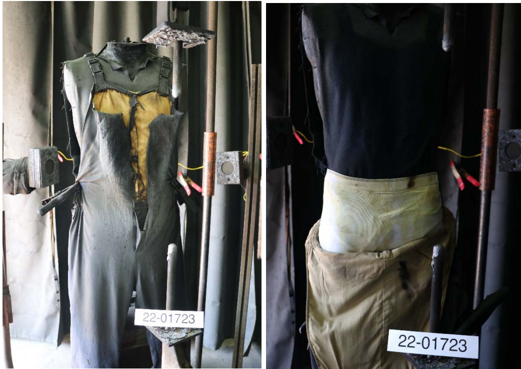
Figure 6.3: Exposure of garment and underlayer garment. (Test# 22-1723A)
