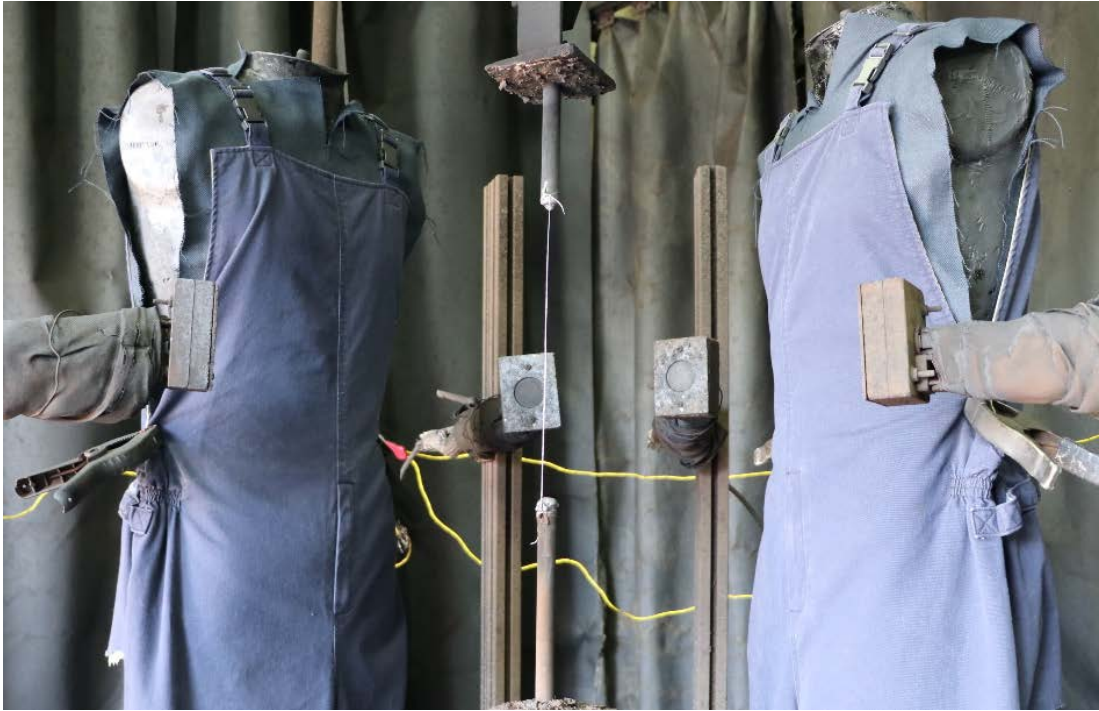
Figure 6.1: Garments as tested before arc exposure.
