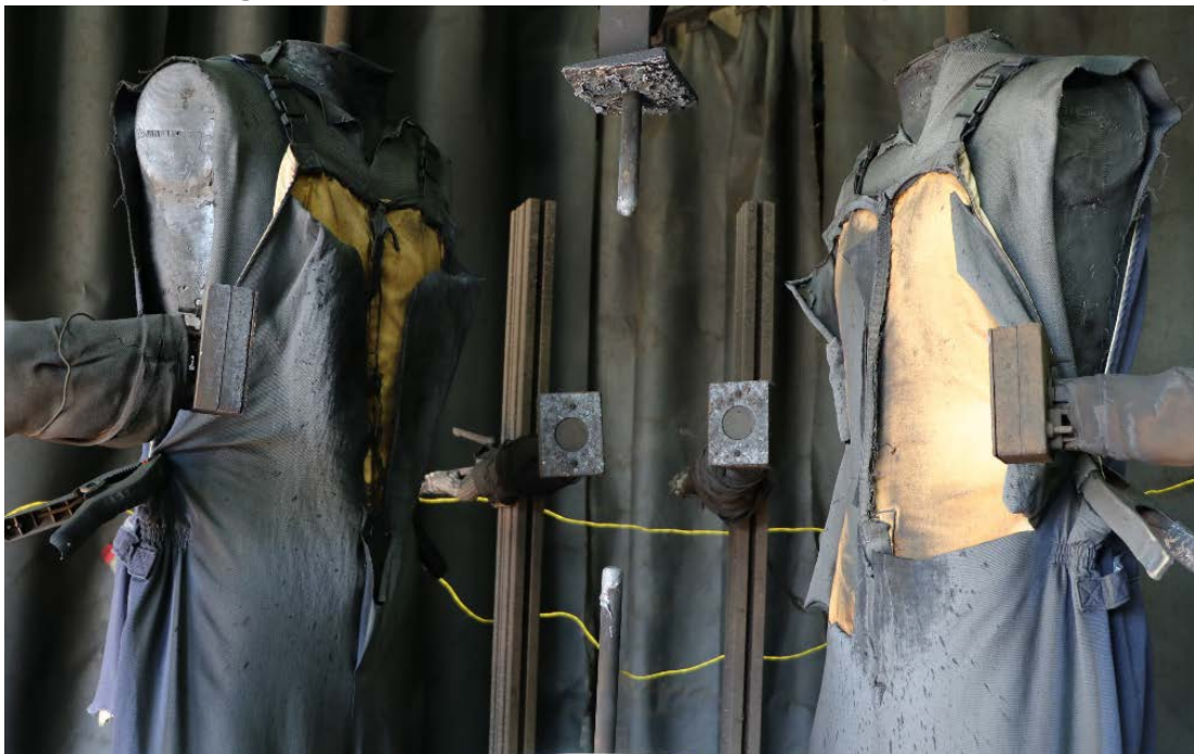
Figure 6.2: Garments after arc exposure. (Test# 22-1723)
