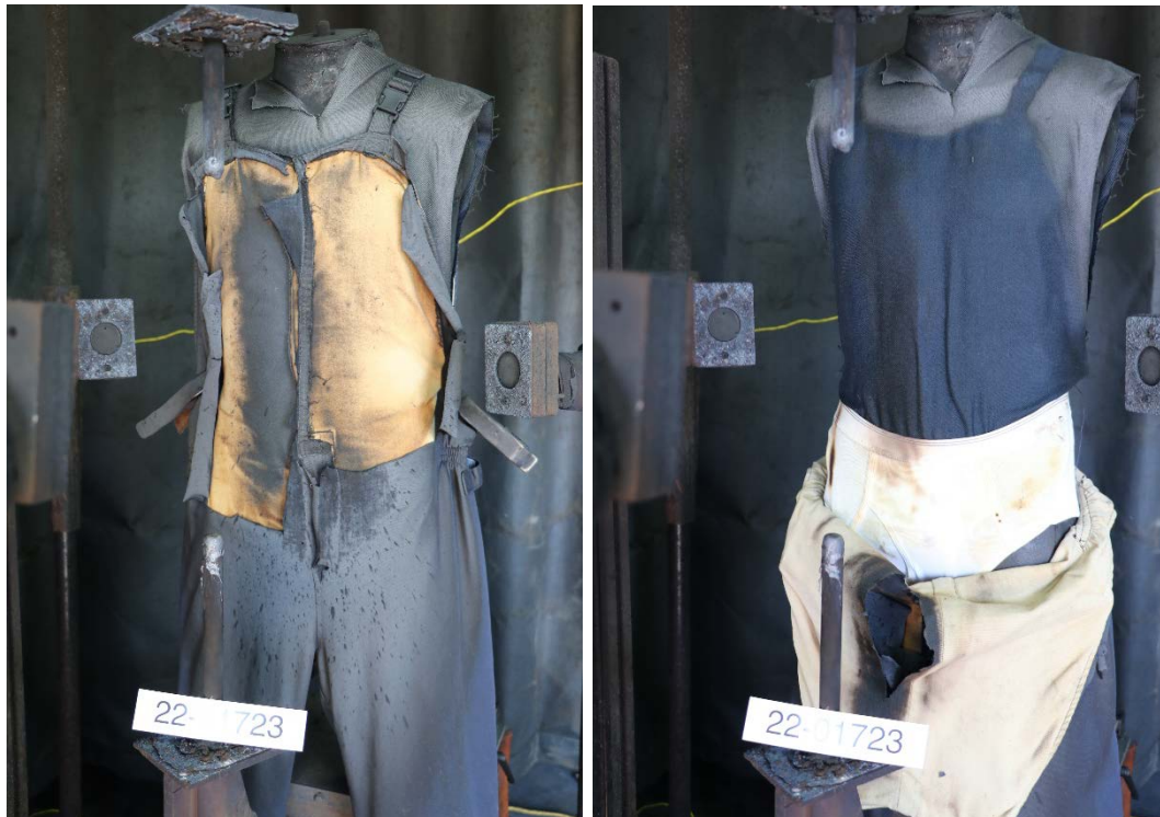
Figure 6.4: Exposure of garment and underlayer garment. (Test# 22-1723B)
