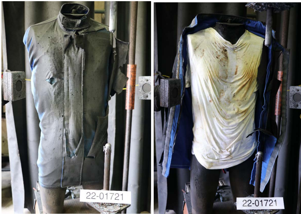
Figure 6.3: Exposure of garment and underlayer garment. (Test# 22-1721A)
