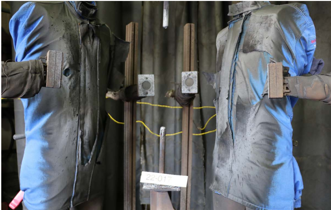
Figure 6.2: Garments after arc exposure. (Test# 22-1721)
