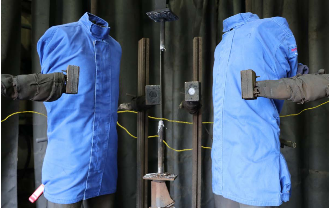
Figure 6.1: Garments as tested before arc exposure.
